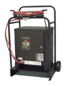
For the loaner type applications there is the LS2/24-28C model that is available with automatic control only. This model comes with a heavy-duty wheeled cart that gives you rugged portability, cable storage, and tie down capability. It is designed to charge from 2 and 24 cells at 28 amps output.. It can be plugged into any 120 volt receptacle. The charger comes complete with 8 ft. of 14/3 AC power cord with a 15 amp molded plug and 10' of DC power cable.
